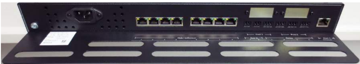
PowerShield Controller LX Rear Panel
