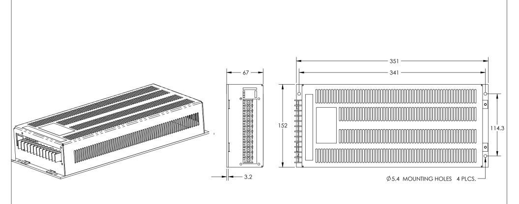
Case material: Aluminum 5052-H32 Finish: clear Iridite as per MIL-C-5541 E Class 3 Typical weight: 2Kg [4.4 lbs.] DIMENSIONS ARE IN MILLIMETERS [Inches] TOLERANCES ON DECIMALS: XXX ± 0.2mm XX ± 0.3mm
