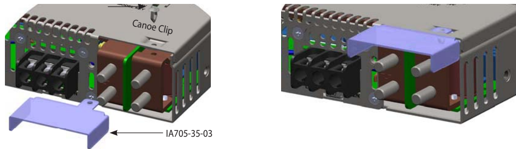
Fig 1.3b Installation of Output Bus-Bars Protection Cover.
