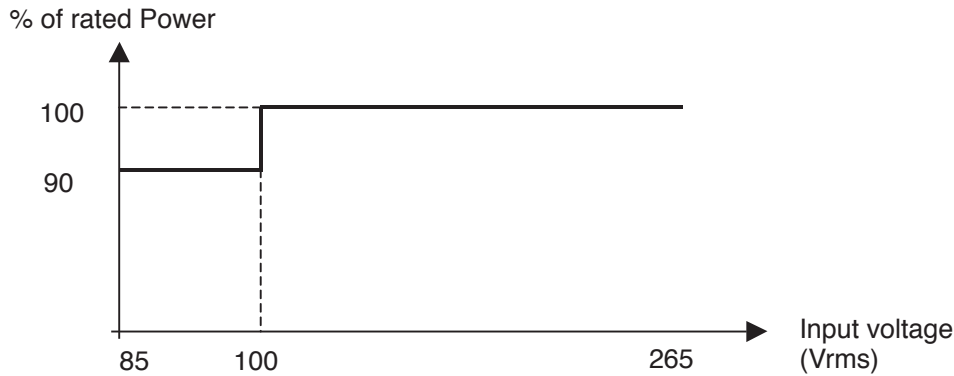
Fig 13-1: Output Power derating at parallel operation
