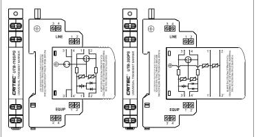
Signal Pair protection with isolated ground connection. Signal wires via terminals LINE side 1,2 and EQUIP side 1', 2'. Signal ground or shield via terminals 3 or 4, grounding via ground tab or DIN rail.
