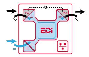
The ECI technology eliminates all single points of failure with full scalability; up to 32 modules in parallel and high efficiency of up to 96% in AC to AC conversion, and above 93.5% in DC/AC conversion, hence reducing operating costs.
