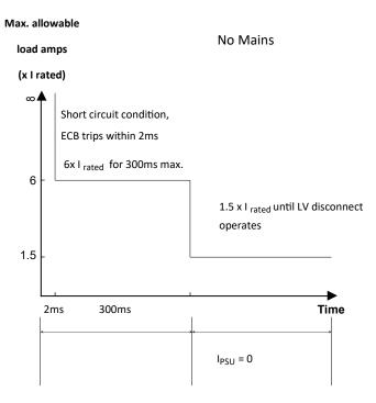
The ECB will operate on overcurrent as above & is also activated for the low voltage disconnect function on mains fail (no input power). It will reset when input power is restored, or can be manually reset by briefly shorting the **BAT**- and **LOAD**- terminals together when there is no input power.
