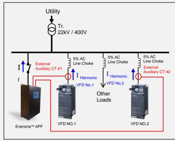
Like all Enersine<sup>™</sup> APF series, the compensation power electronics are packed in compact enclosed modules with forced air cooling designed for wall-mount installations where space is at a premium and harmonic mitigation current is high.
