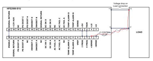
Fig 3.2 Remote Sensing connection diagram
