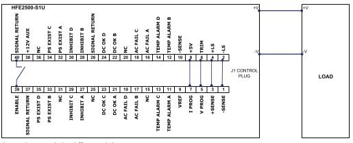
Fig 3.3 Entire rack On/Off control diagram.
