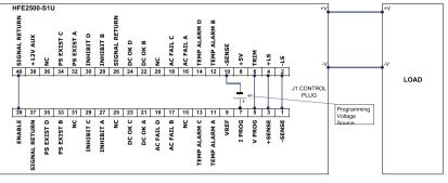
Fig 3.6.1 Output Current programming by External Voltage.
