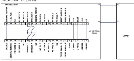
Fig 3.4 individual units On/Off diagram.
