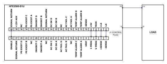
Fig 3.1 Basic connection diagram.
