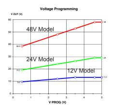
Fig 3.6 Output Voltage programming by External Voltage.
