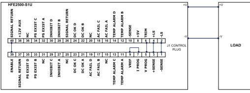
Fig 3.7.1 Output Current programming by PMBus
