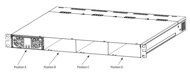
Fig 2.2 Power supply positions
