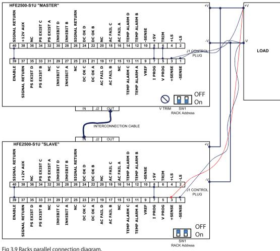
Fig 3.9 Racks parallel connection diagram. \*Note: For PMBUS OPTION in the master rack 1.Disconnect Pin 5&6
