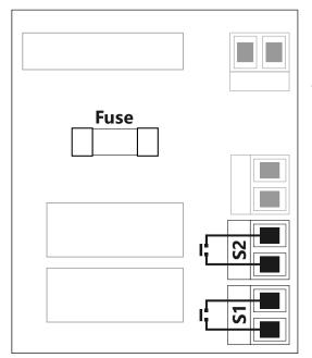
The tripping relays can switch up to 220VDC and 250VAC up to 1A. Normally open, will close if iSTS internal fault.
