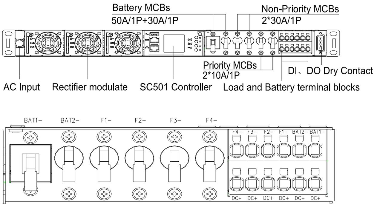
Figure 2-2 Terminals' Position of 1U system
