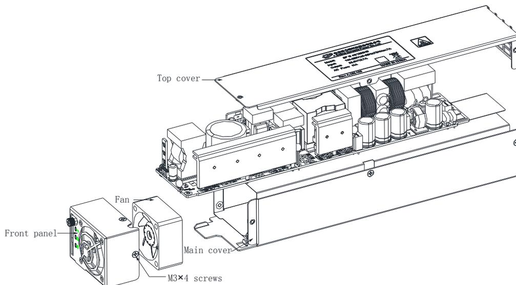
Figure 4-2 Disassembling the front panel
