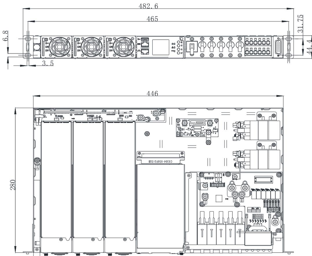
Figure 2-1 Installation Dimension
