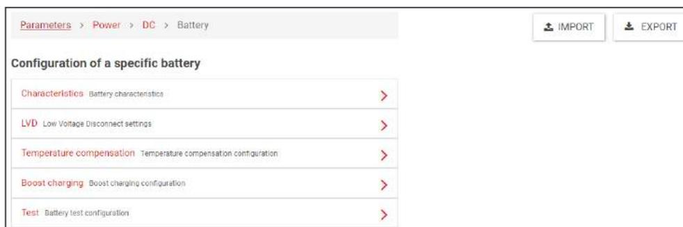
1. **Characteristics:** Displays the battery parameters and configured with default values. User can modify it as per the battery connected in the system.
