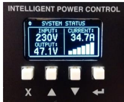
Figure 9: ICM Front Control Interface – System Status Screen
