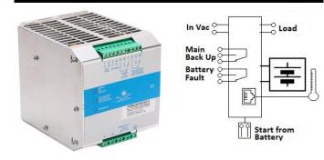
Input: Single-phase 115 - 277 Vac Output Load: power supply 48 Vdc; 5 A Output Battery: charging 48 Vdc; 5 A
