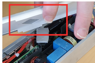
No bulging and warping
