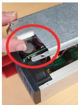
Place the bottom sheet and pay attention to the Formex
