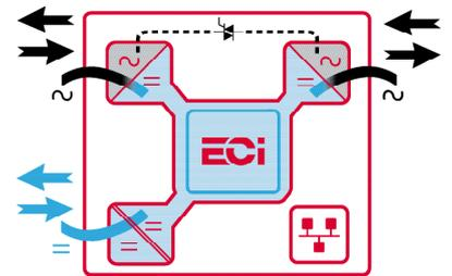
Sierra is also the right choice for **energy management** applications such as grid reinjection, peak shavings, phase balancing or **innovative solutions** based on energy sharing via a DC distribution.
