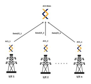
This feature optimizes the collection of information, distributing the reading of the protection devices through different servers, where each server has an instance of Axon Comtrade Server. This allows efficient management of a greater number of devices, managing to scale the service to regional and national networks.
