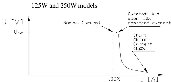
Please note that curves present the current limiting principle only. Exact values and shape of curves varies between different models, refer specification.
