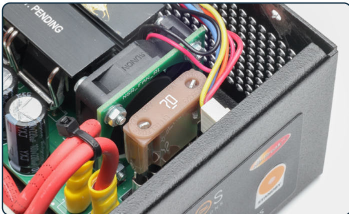
Fuse location. Fuse type and rating varies by model.
