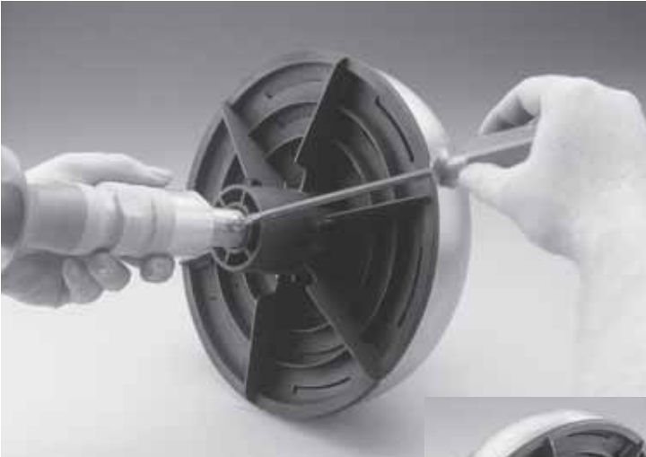
Photo 13: Once the ERITECH® DYNASPHERE has been fitted to the termination coupling, ensure the locking screw is tightened securely.
